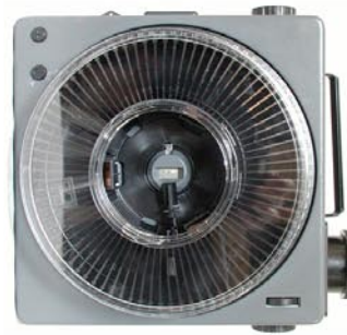
Slide projector 1 of 24 projects film frames 1, 25, 49, ...
