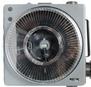
Slide projector 4 of 24 projects film frames 4, 28, 52, ...
