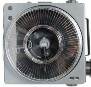
Slide projector 3 of 24 projects film frames 3, 27, 51, ...
